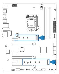
8. Insert the Sabrent ROCKET Q4 NVMe M.2 SSD device pin-side first into the M.2 slot as is illustrated below.
