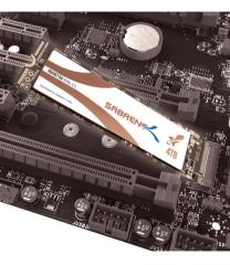
9. Fasten the opposite end of the **Sabrent ROCKET Q4 NVMe** M.2 SSD to the motherboard with the necessary screw or hardware, as is illustrated below.
